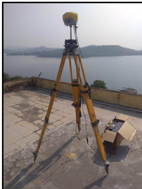
BASE SETUP AT TBM 3
