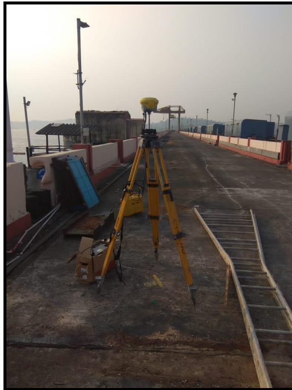
RTK Base setup on OBS MADHUBAN
