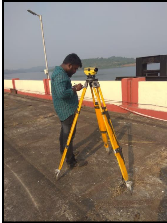
Level transfer from Top of Water Gauge to OBS MADHUBAN
